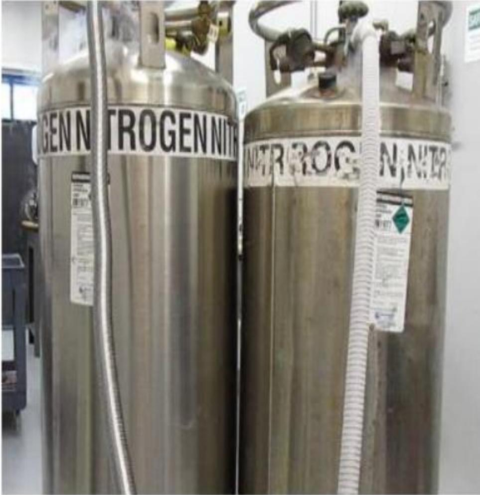
*Vacuum jacketed hose (left) and cryogenic hose (right) transfer liquid nitrogen*
