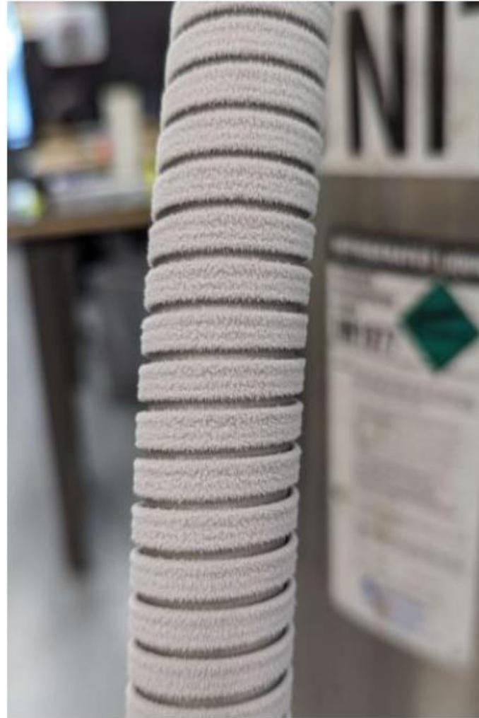
*Cryogenic hose accumulates frost while transferring liquid nitrogen*
